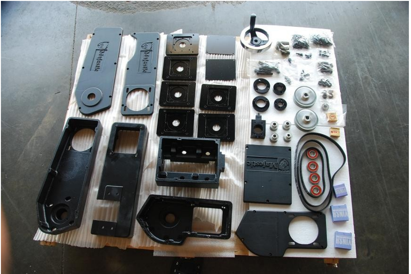
Aluminum castings, thrust bearings, belts, pulleys and hardware included.
